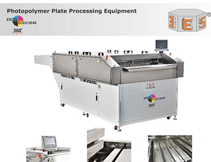
EXCEL-SOLV 3648 is designed as inline high productivity photopolymer plate washing, rinsing and pre-drying equipment, suitable for processing high quality plates up to a maximum size of 920 x 1200 mm.
