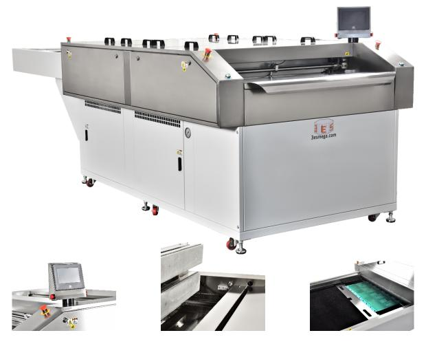
3ES-PROI-WF is designed as inline photopolymer plate washing, rinsing and pre-drying equipment and suitable for processing high quality plates up to a maximum size of 635x762 mm.
