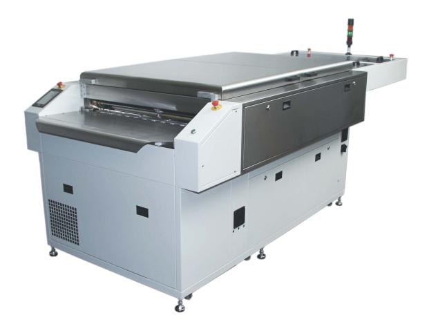
3ES-PROI-FPK is designed as inline high productivity photopolymer plate washing, rinsing, drying and post-exposing equipment, suitable for processing high quality plates up to a maximum size of 660 x 810 mm.
